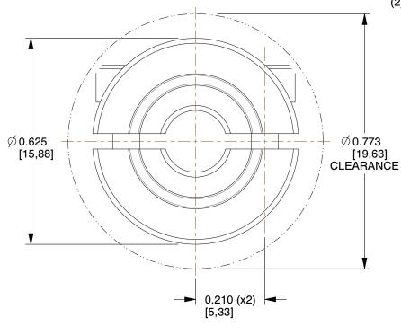
(2) #4-40 Forged Clamp Screws -3/32 in Hex Wrench Size 8 lb-in Seating Torque
