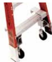
Heavy duty aluminum bracket with 4" castor allows 360° mobility of ladder. Soft rubber wheels are easy on floors; designed to roll over door thresholds. Casters may be used on all 4 legs; order 2 kits for this purpose. Two (2) casters/brackets come with mounting hardware and instructions.
