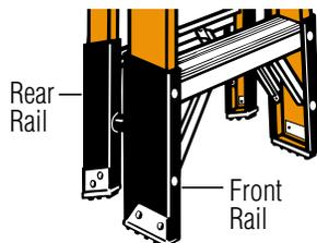
Designed to reinforce. Shields may also be used to repair ladder if rail cracks occur no higher than 3/4" below bottom rivet of bottom step or horizontal and all holes in the rail are intact. Rail shield(s) come with mounting hardware. (1 front and 1 rear kit per stepladder; 2 front kits needed for trestle ladder)
