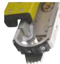
Combination aluminum rail shield bracket and spur-hoop shoe assembly.
