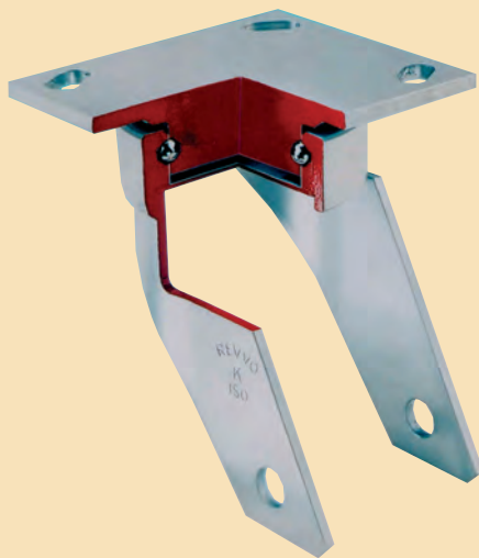
The K Series is a robust fabricated caster featuring a precision machined kingpinless swivelhead containing a full ballrace with hardened-steel balls running in hardened raceways.
