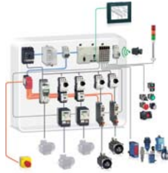
Compact™ / Hardwired / Logic controller / M258™ An excellent performance solution using simple controls architecture...
