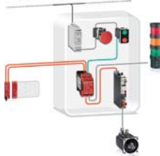
Safety Mat (PL d, SIL 2) Magnetic switches (PL e, SIL 3)
