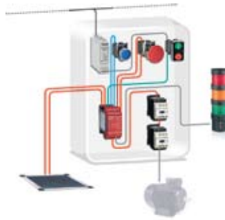
Safety Mat (PL d, SIL 2) Magnetic switches (PL e, SIL 3)
