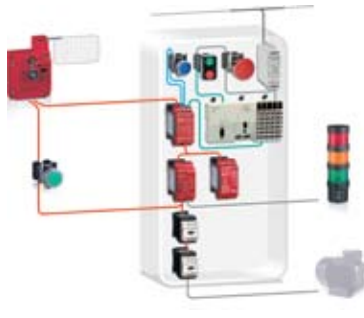
Zero speed detection (PL e, SIL 3) Multifunction (PL e, SIL 3)
