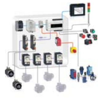
Compact / CANopen™ / Logic controller / M238 Simple setup with easy installation and maintenance...
