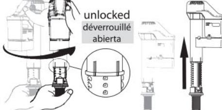
Turn top of new valve counterclockwise to unlock and pull up to fully extend.
