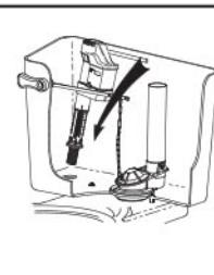
Place locked valve in tank at one of angles shown in 4b.
