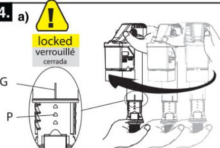
Twist upper half of valve clockwise to lock (snap).
