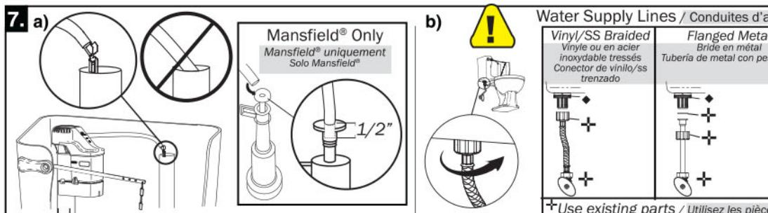
**Attach to overflow tube with metal clip.**
