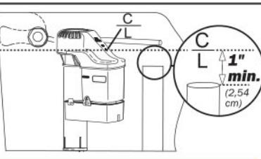
Verify critical level (C/L) is 1" above overflow tube. Code requirement.
