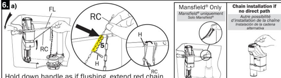
**Hold down handle as if flushing, extend red chain (RC) to flush lever (FL) hole with no slack and direct path.** Note chain link closest to hole, count back 5 links and attach hook (H). Attach to flush lever.
