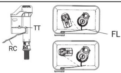
Attach red chain (RC) to tilt cup tab (TT) on the side which allows direct path to flush lever (FL).
