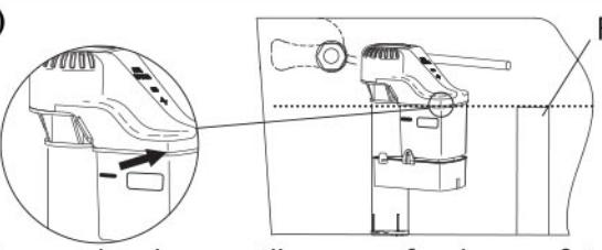
Press valve down until corner of red cover & top of flush valve (FV) line up. Note: If tower style flush valve (TS), match fill valve water line to water line marked in tank (stain line).
