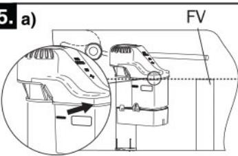
Verify corner of red cover and top of flush valve (FV) line up.
