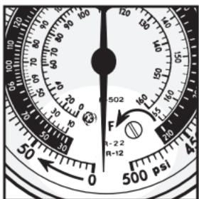
Turn recal screw counterclockwise. Pointer turns clockwise.
