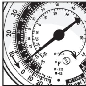
Turn recal screw clockwise. Pointer turns counter-clockwise.
