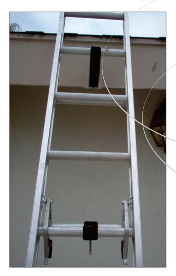
Your LSD Kit provides you with two stability belts - one for the device and one for securing the mid lock on your extension ladder. After extending to the desired heights, wrap one of the belts around two of the adjoining rungs near the mid lock section.
