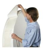
In just three simple steps your purge dam is complete! The illustration is a large bore pipe, 24" in diameter.
