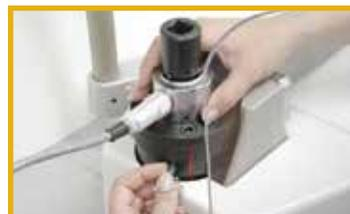
Quick Release Pins make changing transducers a snap
