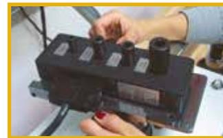
4 in 1 Transducer Kit with Mounting Adapter.
