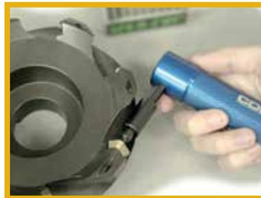
Prevents premature wear of carbide inserts and damage to cutter head due to improper clamp load.
