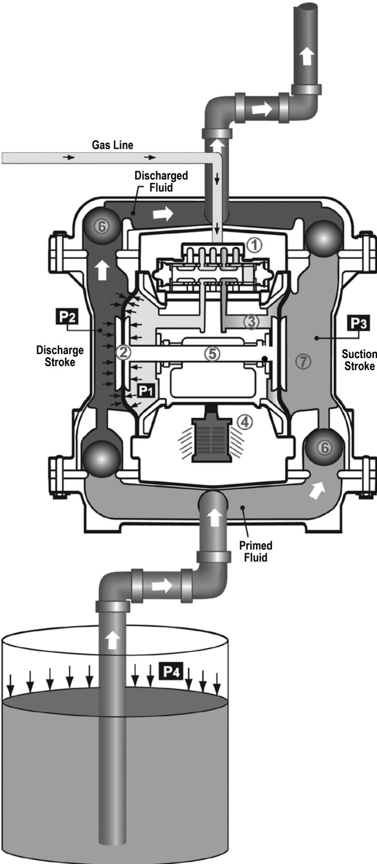
Gas-Operated Double Diaphragm pumps are powered by compressed gas, nitrogen or natural gas.
