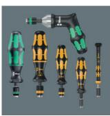
Wera torque screwdrivers. With a factory pre-set torque value set to the smallest scale value. For all applications, where the same constant torque and repeat accuracy are required. The torque can be changed with an extra tool within the measuring range (re-calibration kit can be ordered with the code number 05137001001). Afterwards you can check the set value using an off-the-shelf torque tester.
