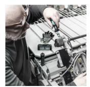
Many screws - particularly in assembly and maintenance applications - have to be tightened with controlled torque to ensure the dependability of the screw connection and/or to avoid damage to the screw or work piece. Wera's adjustable torque screwdrivers are the ideal tool for this. They feature a torque range of 0.3 Nm to 8.8 Nm, two different handles, measurement accuracy of  $\pm$  6 % and Rapidaptor technology for rapid bit change.
