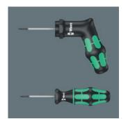
Wera torque-indicators have been factory pre-set to values recommended by leading carbide manufacturers. These tightening values relate specifically to the size of the TORX®, TORX PLUS® or hexagon socket screw. Torque indicators ensure safe and loosening easy of screw connections. Precision :  $\pm$  10 %
