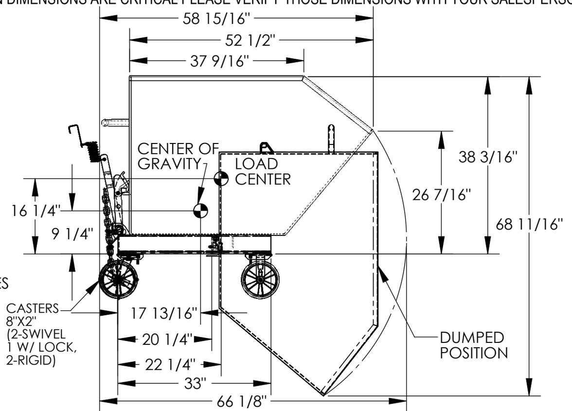
\*\*\* UNIT MUST BE SECURED TO THE FORK TRUCK WHEN DUMPING \*\*\*
