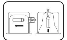
(2) Remove the existing fluorescent lamps from the fixture and dispose of them properly based on local regulations.
