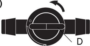
Turn refill adjuster dial (D) counter clockwise to fully closed.
