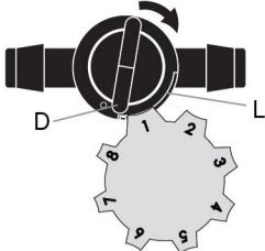
Locate adjuster key setting from Fit Chart below and place on ledge (L) as shown. Adjust amount of refill water by turning adjuster dial (D) clockwise until it contacts adjuster key.
