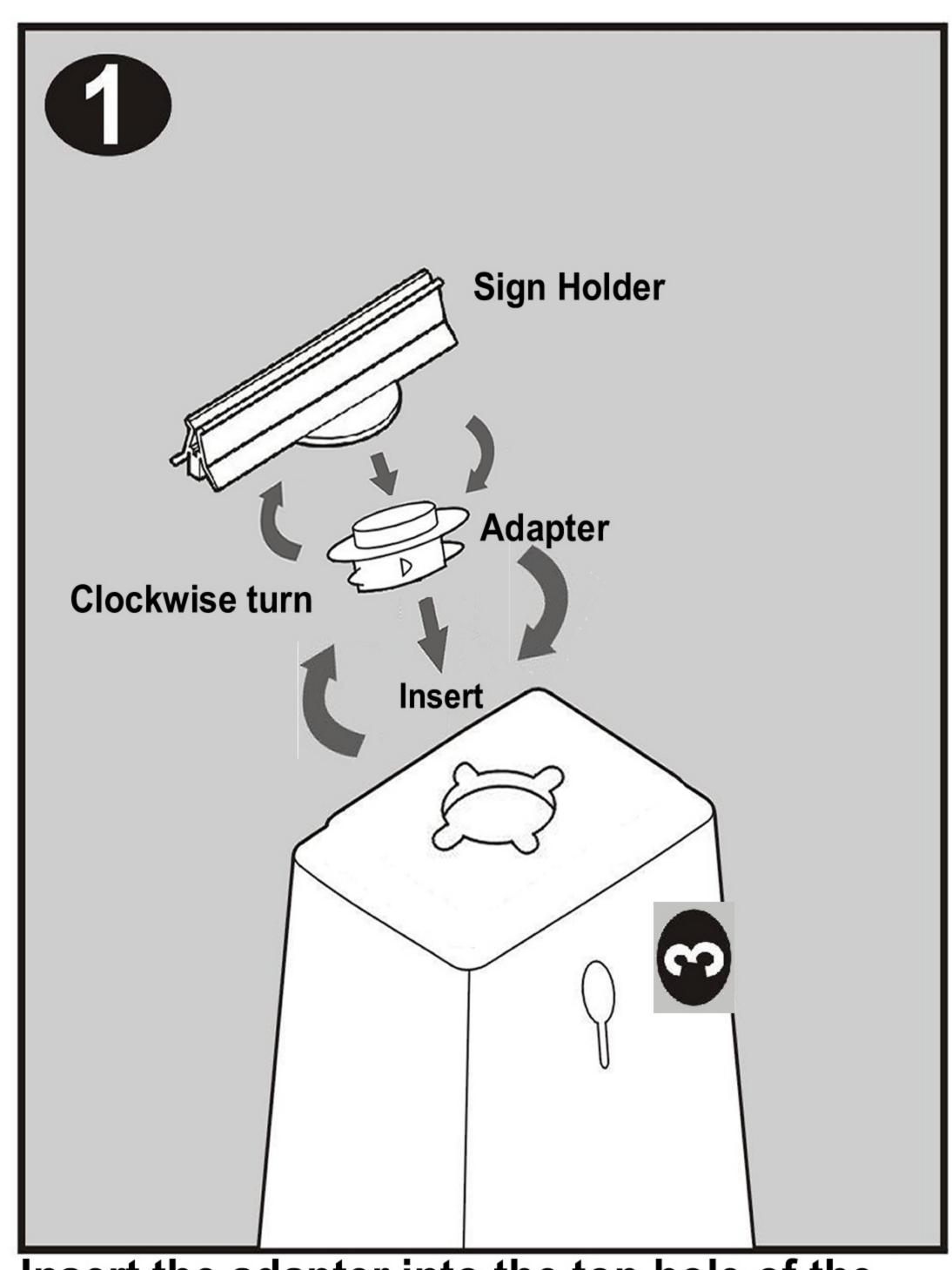
Insert the adapter into the top hole of the cone. Insert the sign holder into the adapter by aligning the engagement points of both items. Turn the sign holder and adapter approximately 1/4 turn clockwise to lock the assembly into position.
