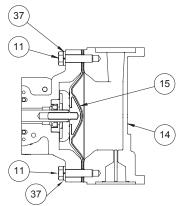
**Diaphragm Orientation**Install diaphragm and spacer
