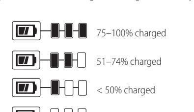
To actuate the fuel gauge, press and hold the fuel gauge button. A combination of the three green LED lights will illuminate designating the level of charge left. When the level of charge in the battery is below the usable limit, the fuel gauge will not illuminate and the battery will need to be recharged.
