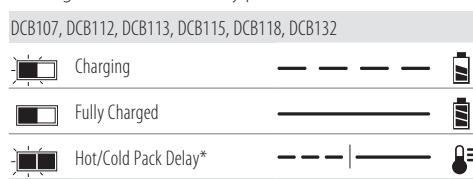
**\*DCB107, DCB112, DCB113, DCB115, DCB118, DCB132:** The red light will continue to blink, but a yellow indicator light will be illuminated during this operation. Once the battery pack has reached an appropriate temperature, the yellow light will turn off and the charger will resume the charging procedure.
