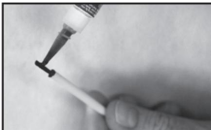
2. Insert stripped end into eye. Fish tape must bottom-out in eye, and fiberglass end must extend completely to the edge of eye hole.
