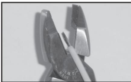
2. Strip outer orange nylon jacket exposing inner fiberglass. Use 45-895 Strimaster® Wire Stripper with LB-1156 blade. Or, safely strip away nylon with razor blade.
